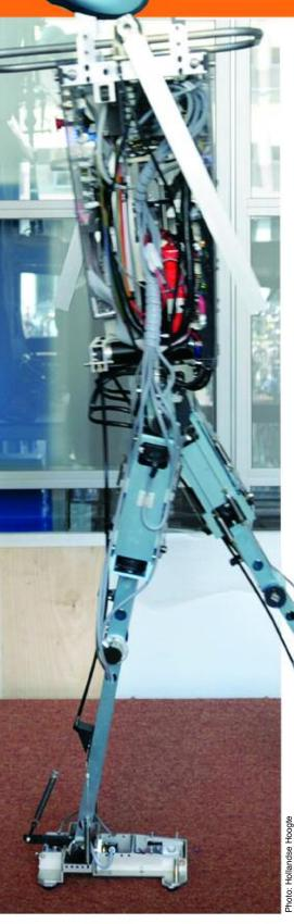
Consider Denise, a two-legged robot that walks more like a person than a machine. Martijn Wisse in the Biorobotics Laboratory in Delft developed Denise. Like us, she falls forward and then catches herself with each step.
