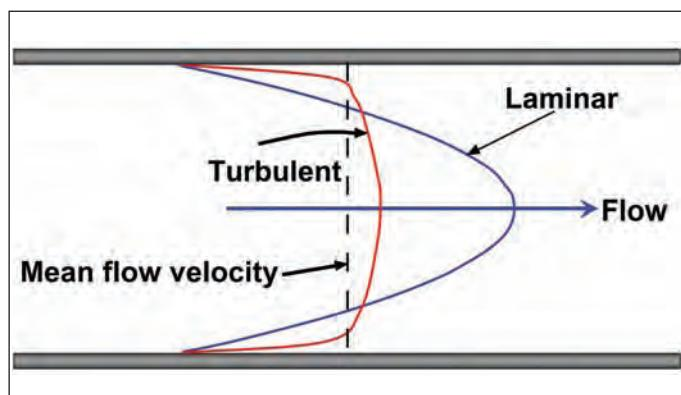
Figure 1: Flow Velocity Meters Work Best on Flows with Turbulent Profiles (Red Line).
