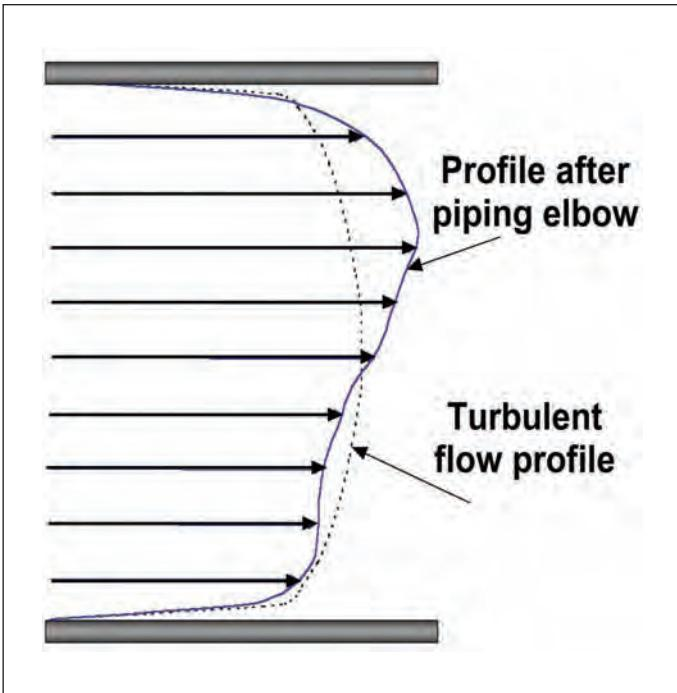
**Figure 2: Pipe Fittings Near the Flowmeter can Distort the Flow Profile, Requiring Straightening Devices.**
