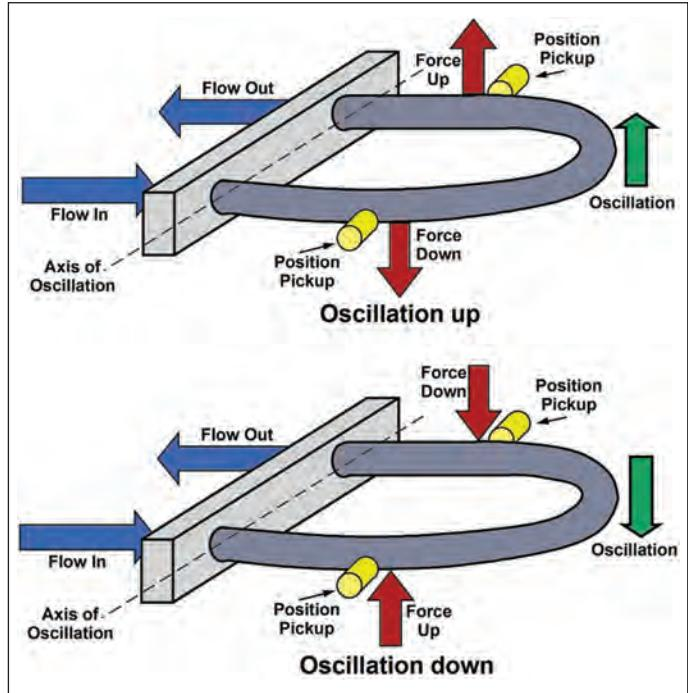
**Figure 12: Principle of Operation for Coriolis Flowmeters**
